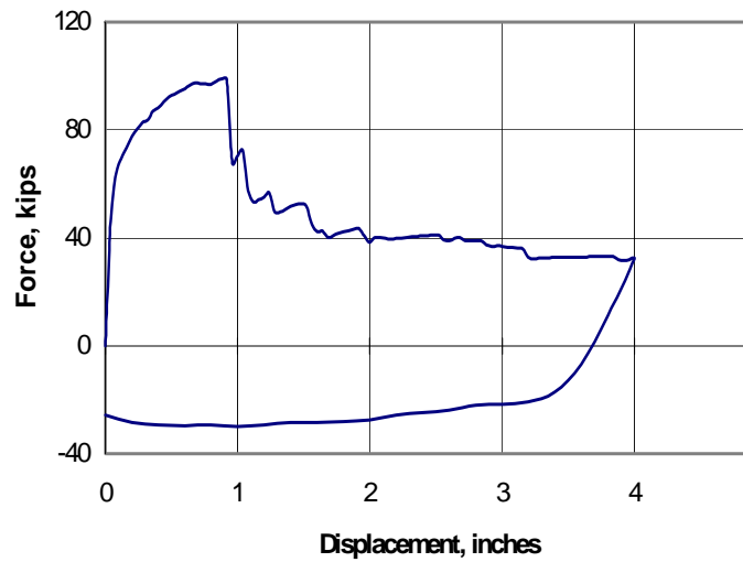
(a) Strong Infilled Frame (Model #2)
